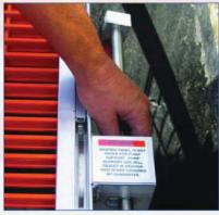
Grasp the hold open arm with the red latch facing down. Place the end of the hold open arm through the slot in the slide angle that is located on the side of the Retro-Grate<sup>TM</sup> structure. Pull the hold open arm assembly through the slide plate angle all the way to the lower clevis located below the pivot side support bracket.
