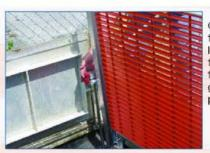
Grasp the spring loaded lifting handle and pull the Retro-Grate™ into the open and upright position. If the unit is installed properly, the red latch should move into a locked position beneath the slide angle and the grating structure cannot be lowered. If the latch does not move into the locked position, consult the factory. To lower the Retro-Grate™, grasp the lifting handle with one hand and with the other hand, simply pivot the red latch upward and lower the unit.
