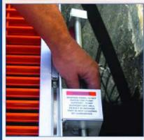
Grasp the hold open arm with the red latch facing down. Place the end of the hold open arm through the slot in the slide angle that is located on the side of the Retro-Grate™ structure. Pull the hold open arm assembly through the slide plate angle all the way to the lower clevis located below the pivot side support bracket.
